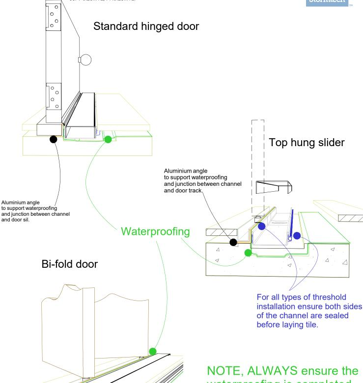
NOTE, ALWAYS ensure the waterproofing is completed before laying the Stormtech.
