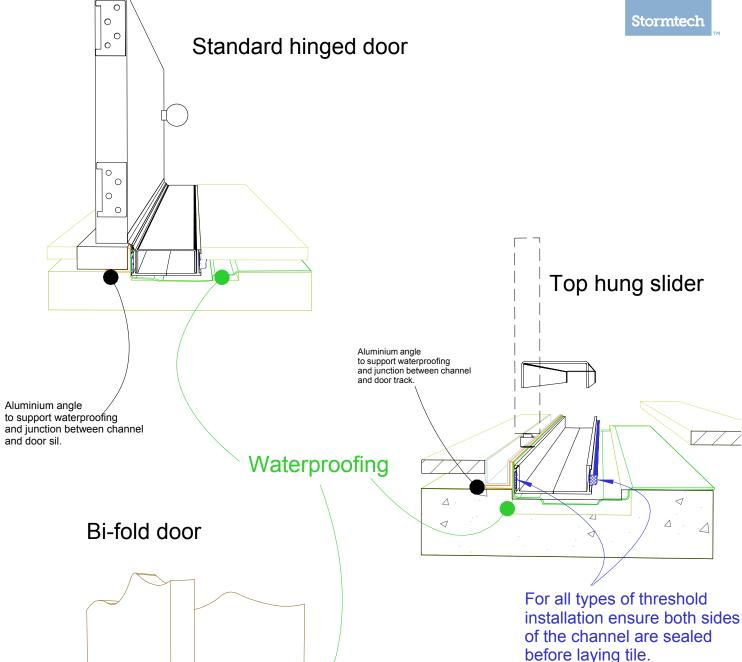
NOTE, ALWAYS ensure the waterproofing is completed before laying the Stormtech.
