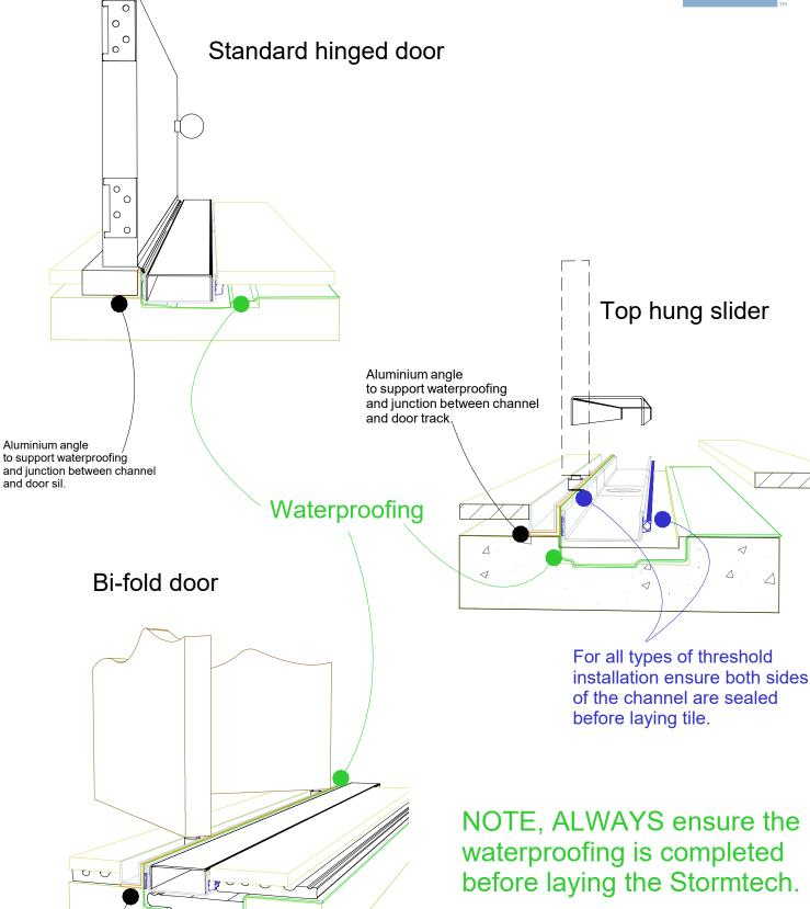
Aluminium angle to support waterproofing and junction between channel and door track.
