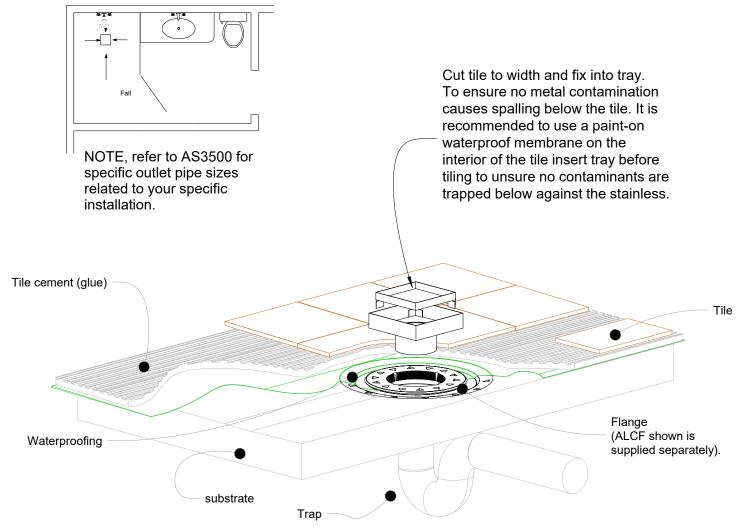
NOTE, this method requires the drain body to be above and separate from the waterproofing. Ensure the floor falls to drain are at least 1:80
