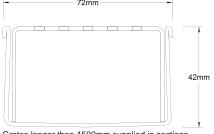
Grates longer than 1500mm supplied in sections. Tile Inserts longer than 1200mm supplied in sections. Channels over 3000mm supplied in sections with joiner.
