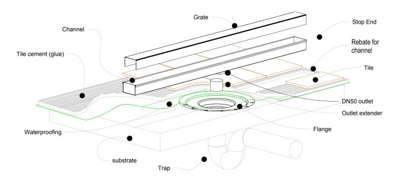
NOTE, this method requires the channel system to be ABOVE and SEPARATE from the WATERPROOFING.
