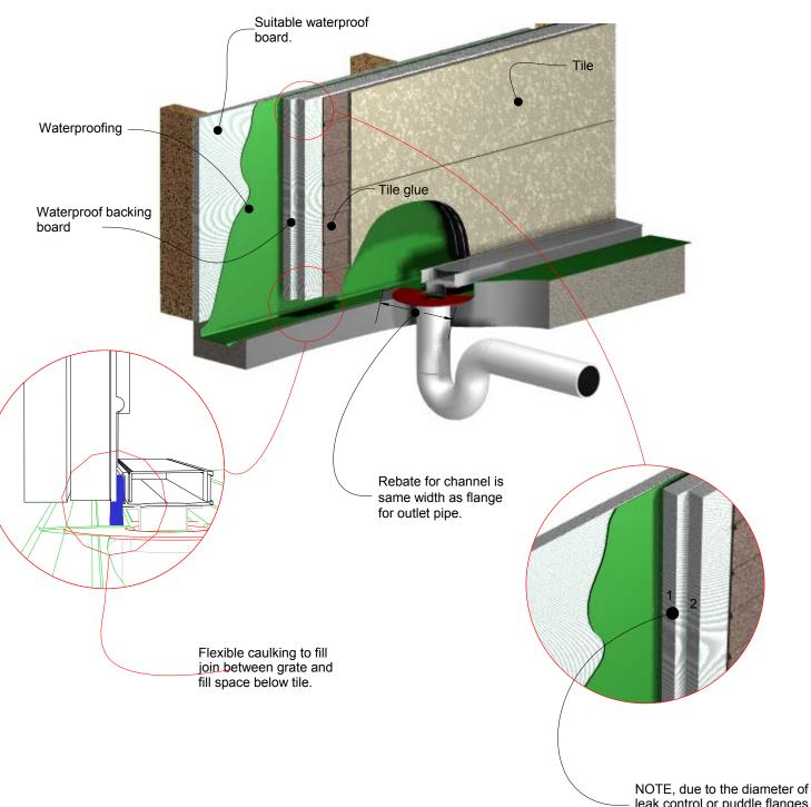
NOTE, due to the diameter of leak control or puddle flanges up to two layers of waterproof backing board or villa board may be needed to pack out wall before tiling.
