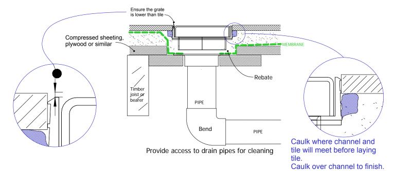
When 100G20 is running perpendicular to joist/bearer
