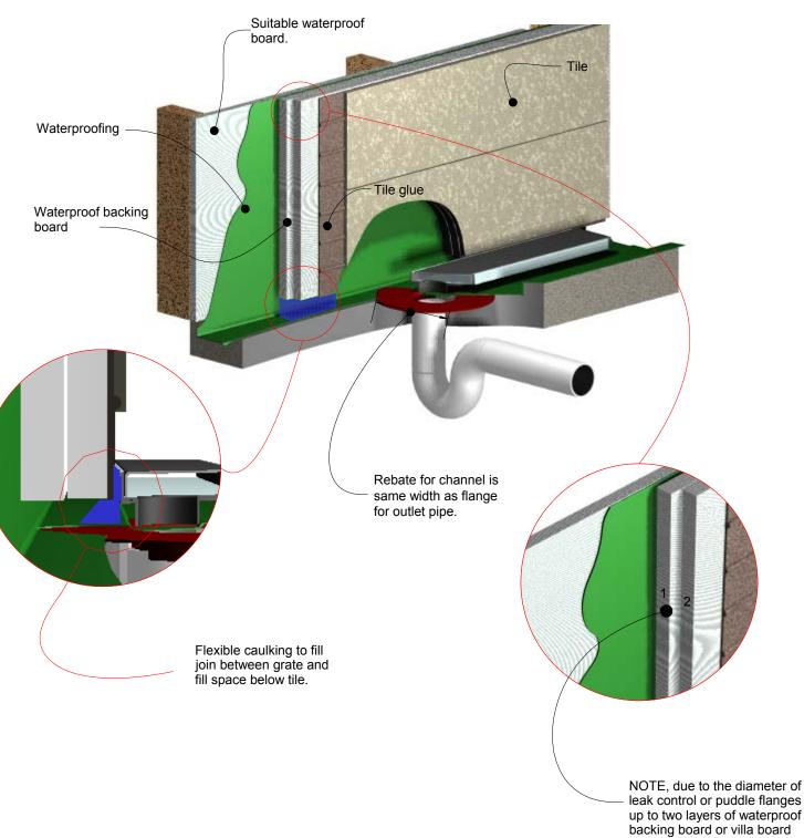
leak control or puddle flanges up to two layers of waterproof backing board or villa board may be needed to pack out wall before tiling.
