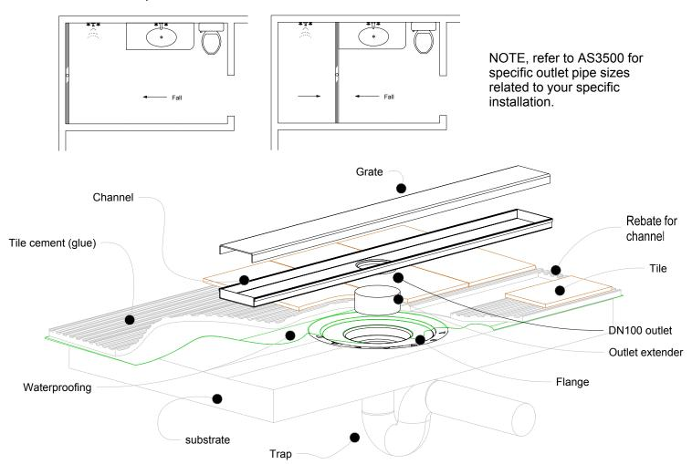
NOTE, this method requires the channel system to be ABOVE and SEPARATE from the WATERPROOFING.
