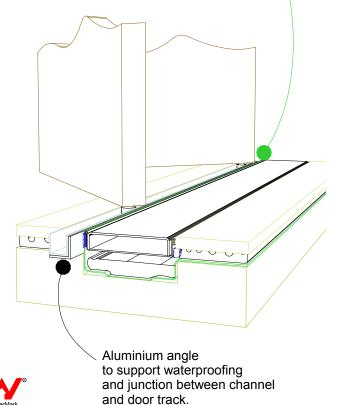
For all types of threshold installation ensure both sides of the channel are sealed before laying tile.
